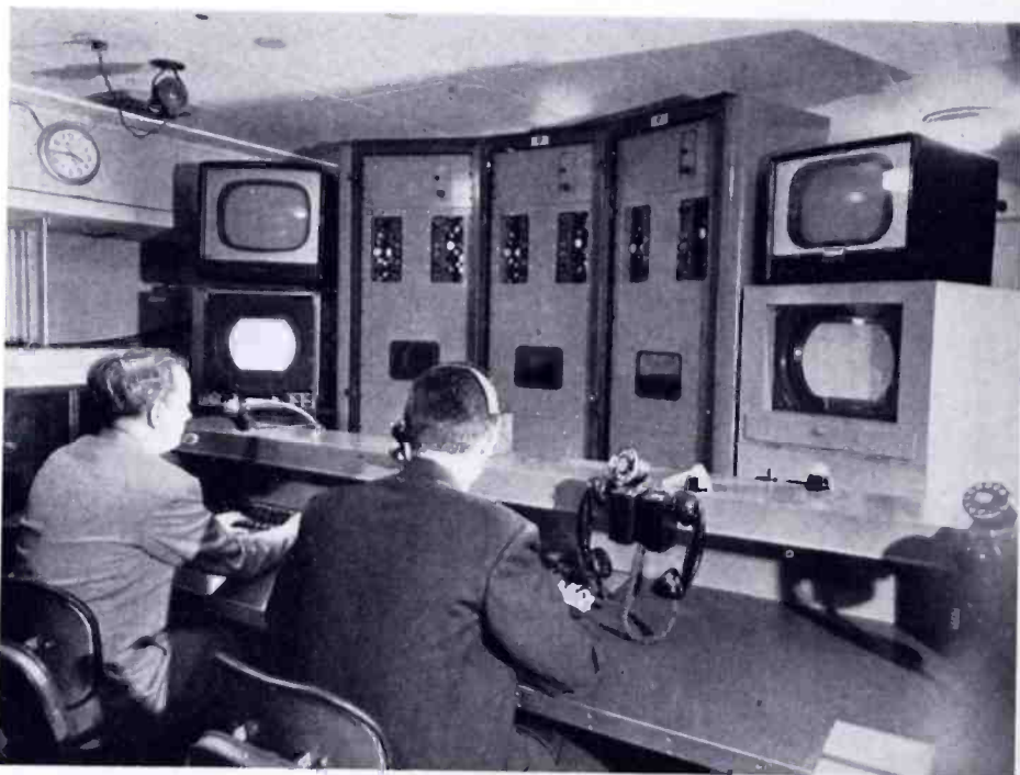
Fig. 5—Photograph of arrangement of monitors with technical and program directors' console.
